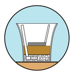
7. Insert the PVC fill tube onto Reservoir. Trim secured fill tube to desired height.
