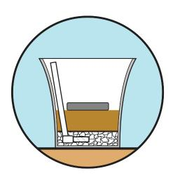
5. Add a base layer of soil. 6. Place Reservoir tank on top of base layer of soil in a level position.
